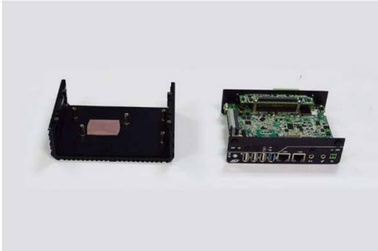
2. Ensure thermal pad is in place where the CPU is located or paste the thermal pad back on the CPU thermal block.
