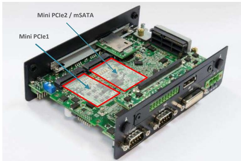
2. Insert mini PClecard or mSATA module from 45 degree direction.
