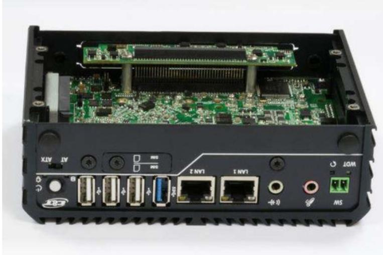
5. Fasten the three screws (M3x5L) and two copper stud (M3x11L) to lock the system body with top cover.
