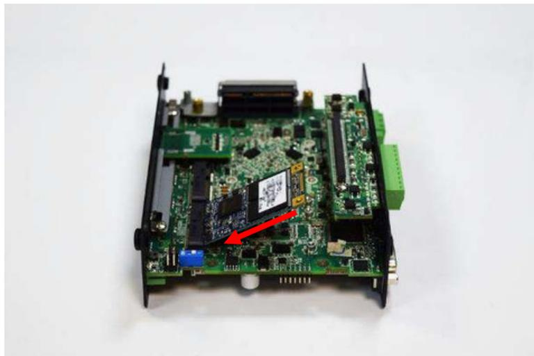
3. Press the mini PClecard or mSATA module down and lock it with two screws (M2x3.7L).
